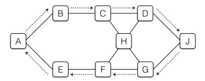
The machine A has initiated a TCP connection to machine J. As it turns out, all packets from A to J happen to follow the path indicated by the right-facing dotted arrows, and all packets from J to A happen to follow the path indicated by the left-facing dotted arrows. Machines A and J use modern TCP software and do not have any special defenses against attack.
