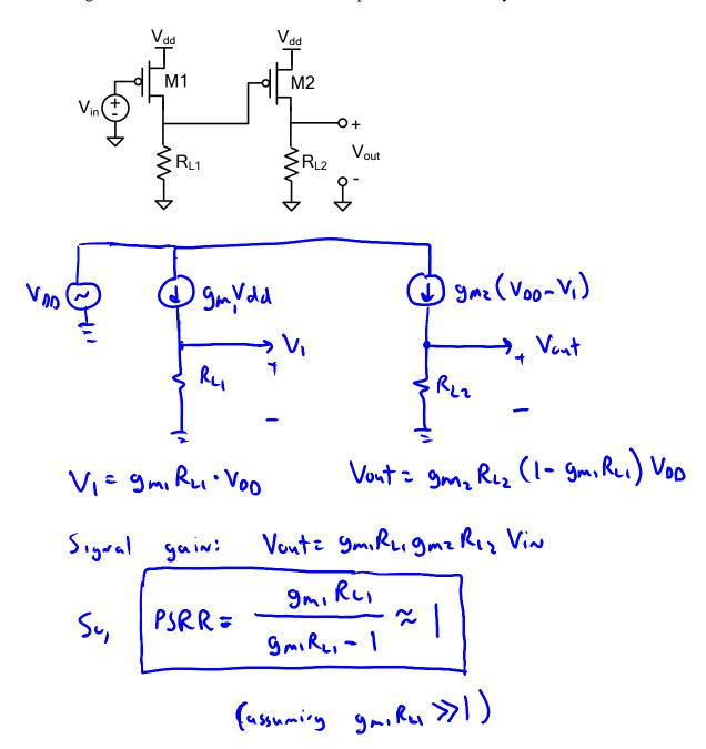
b) (5 pts) Your co-worker Pat says that she can fix the PSRR problem with the design from part a) by changing just one of the two common-source stages and without using differential amplifiers. Is Pat right? If so, which stage would you change, and how would you change it? If not, why not?
